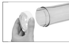
4. Re-insert the Disc/Tip Adapter back on to the Dough Barrel and turn clockwise into the lock position.
